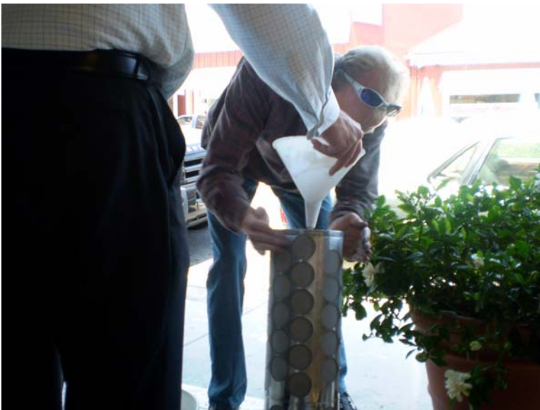
Figure 3-4. Pouring Tonsil into Test Filter
