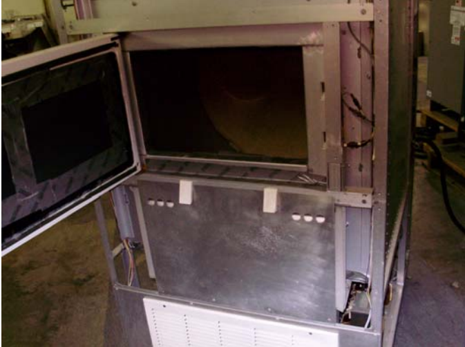
Figure 4-15. Microwave Dryer with Open Door
